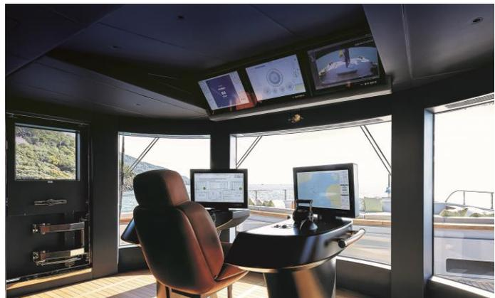
The supply includes integrated navigation with certified X-band radar and electronic cartography, tourist cartography, Seastema conning display, certified log and echo sounder, AIS, DGPS, REG-Code class GMDSS communications.
